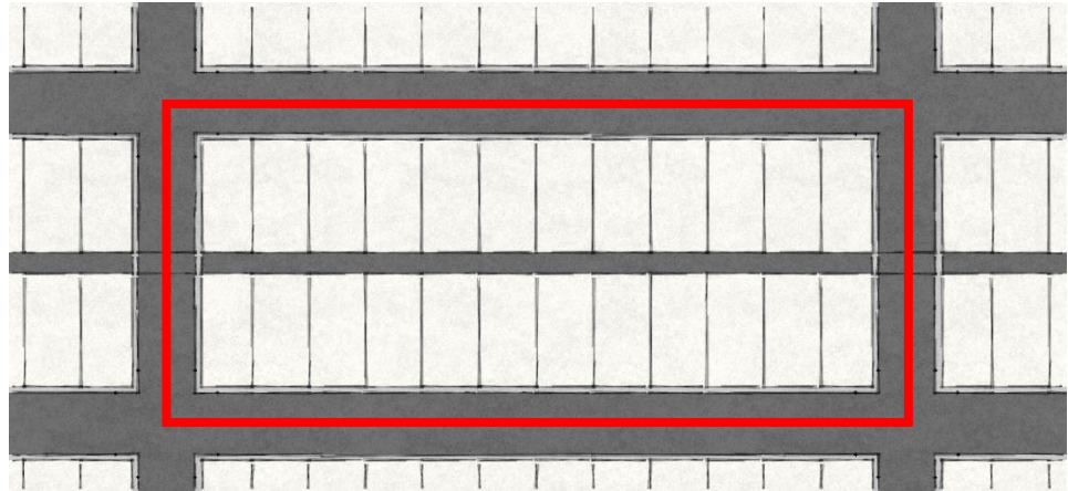
Figure 60.5.1: maximum block dimensions as per 60.5.2(1)(a) of this section.
